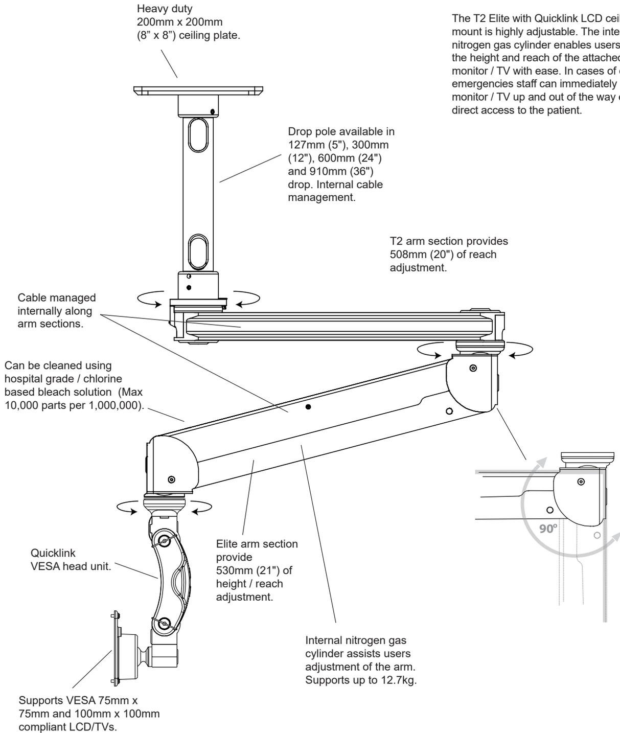
The T2 Elite with Quicklink LCD ceiling mount is highly adjustable. The internal nitrogen gas cylinder enables users to adjust the height and reach of the attached LCD monitor / TV with ease. In cases of clinical emergencies staff can immediately swing the monitor / TV up and out of the way enabling direct access to the patient.
